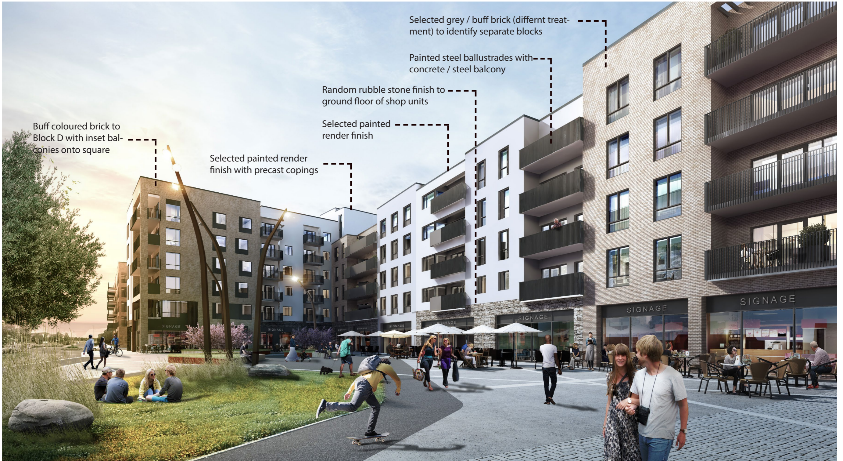
Elevation to new District Square showing brick / metal railings and local stone cladding to ground floor retail units
