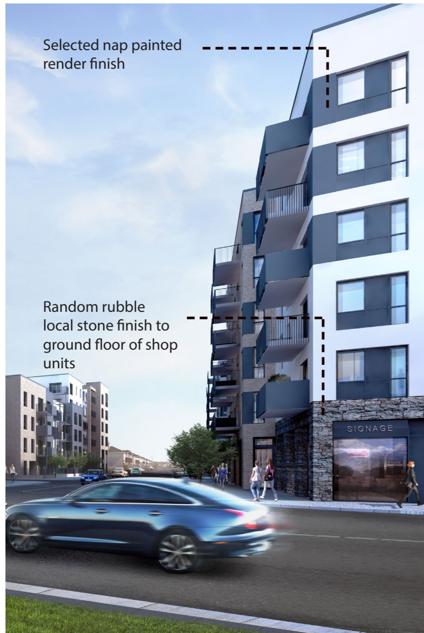
Elevation of Block D to new District Square showing coloured render finish, metal railings and local stone cladding to ground floor retail units
